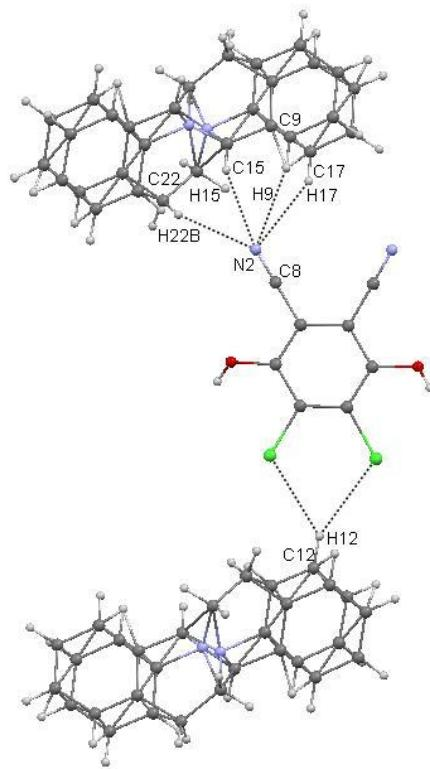
**Figure S1.** X-ray Crystallography: Interactions between: (a) DDQ units and (b) DDQ:THIQ units in complex **4**. Significant H-bonding parameters are given below
