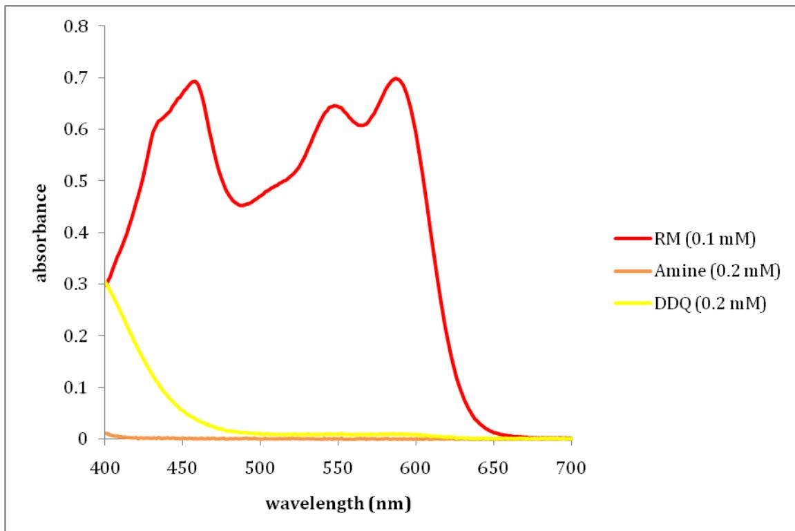
Solutions of 2-phenyl-1,2,3,4-tetrahydroisoquinoline and DDQ were made with nitromethane (0.2 mM) and UV-visible spectra (400 – 900 nm) were recorded at room temperature. The solutions were combined in a 1:1 ratio to give the reaction mixture (0.1 mM) and UV-visible
