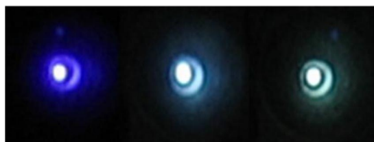
Fig. 7 Photographs of SalHBP under 9.8 kbar (left), 25.2 kbar (middle), and 51.1 kbar (right). The diameter of the light spot is about 300 \mu\text{m} . Centers of light spot are overexposure. Reproduced from ref. [16a], with permission of the American Chemical Society.
