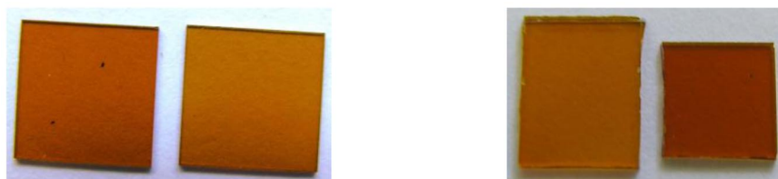
Fig. 1 (a) Left: 650-nm-thick film of \text{Bi}_{1.8}\text{Lu}_{1.2}\text{Fe}_{3.6}\text{Al}_{1.4}\text{O}_{12} on a \text{Gd}_3\text{Ga}_5\text{O}_{12} (GGG) substrate; Right: 1150-nm-thick film of ( \text{Bi}_{1.8}\text{Lu}_{1.2}\text{Fe}_{3.6}\text{Al}_{1.4}\text{O}_{12} + 20 vol % co-sputtered \text{Bi}_2\text{O}_3 ) on a GGG substrate (both films are as-deposited); (b) Left: 1030 nm ( \text{Bi}_2\text{Dy}_1\text{Fe}_4\text{Ga}_1\text{O}_{12}:\text{Bi}_2\text{O}_3 24 vol %) on glass, after 2 h @ 580 °C, Right: 1080 nm \text{Bi}_2\text{Dy}_1\text{Fe}_{4.3}\text{Ga}_{0.7}\text{O}_{12} on GGG, after 1 h @ 700 °C.
