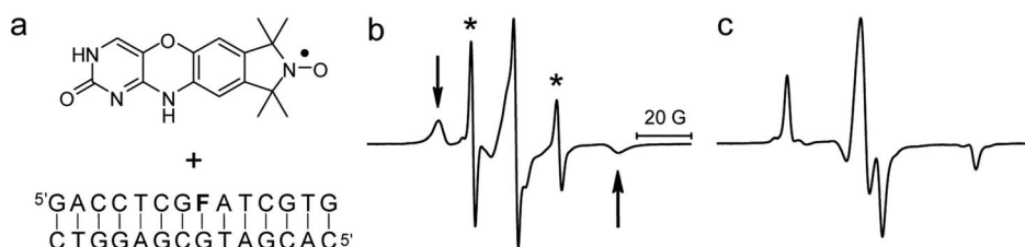
Fig. 6 Binding of the spin label \zeta to an abasic site (F) in duplex DNA (a), monitored by EPR spectroscopy at 0 °C (b) and -30 °C (c). The peaks associated with binding of the spin label to the abasic site are identified with arrows, and the peaks arising from unbound \zeta are labeled with a star.
