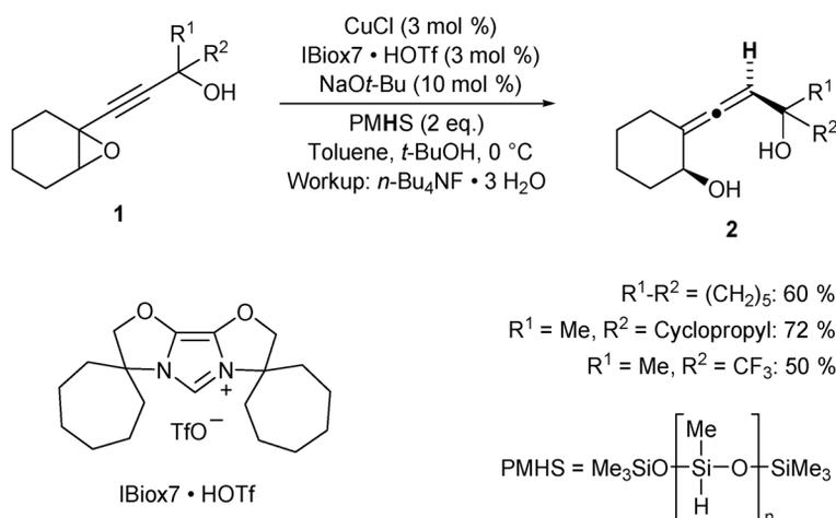
**Scheme 1** Copper-catalyzed  $\text{S}_{\text{N}}2'$ -reduction of propargyl oxiranes **1**.
