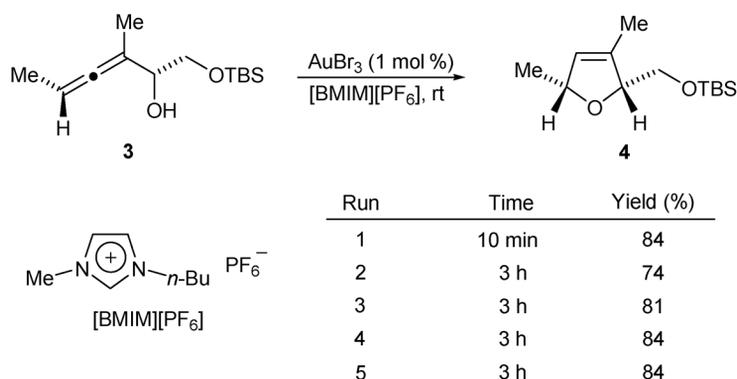
**Scheme 3** Gold-catalyzed cyclization of  $\alpha$ -hydroxyallene **3** in the ionic liquid [BMIM][PF<sub>6</sub>].
