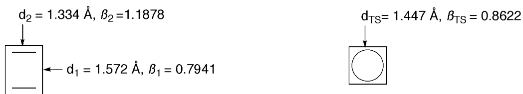
Scheme 7 Equilibrium (B3PW91/6-31G**) and transition state (CASSCF/cc-pVTZ) geometries of cyclobutadiene in the singlet state [25,26]. The variable resonance integrals values given in reference \beta units are obtained from empirical formulae of ref. [24].
