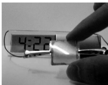
Fig. 10 Flexible plastic battery totally composed of organic radical polymers.
