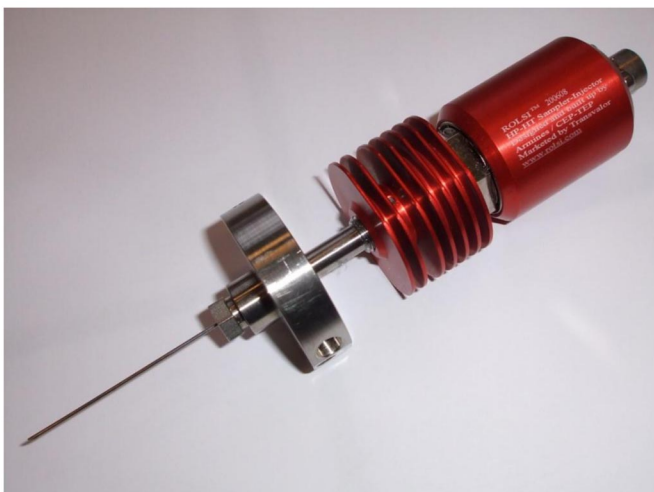
Fig. 5 Electromagnetic ROLSI sampler.
