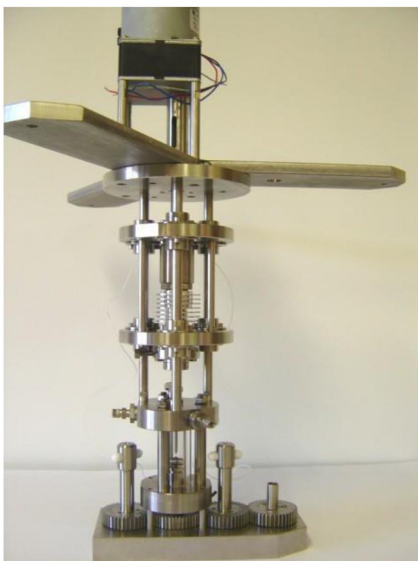
Fig. 4 Equilibrium cell with a movable ROLSI sampler.
