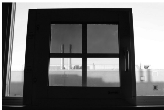
Fig. 5 “Smart window” prototype with four 30 \times 30 \text{ cm}^2 panes.
