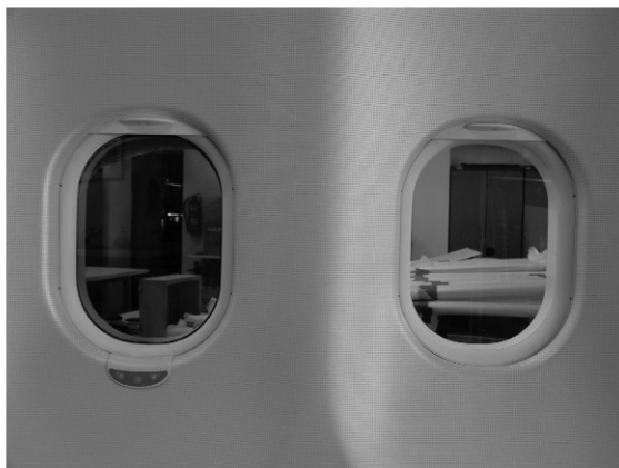
Fig. 6 EC-based airplane window prototypes.
