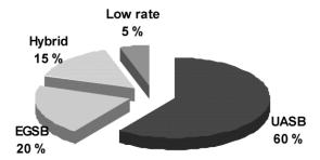
Fig. 1 Distribution of modern anaerobic WWTPs (total: 20) constructed in Russia during 1998–2007 with regard to reactor type (updated from [6]).
