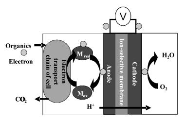
Fig. 3 Schematic representation of MFC.
