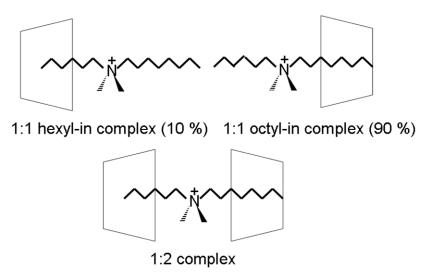
Fig. 7 Structures of 1:1 and 1:2 complexes between  $\alpha$ -CD and HDOAB [31].
