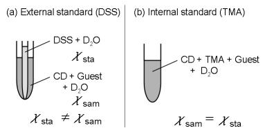
Fig. 2 External and internal standard methods for the chemical shift determination: DSS = sodium 4,4-dimethyl-4-silapentanesulfonate, TMA = tetramethylammonium chloride, and  $\chi$  = volume magnetic susceptibility.
