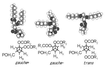
Fig. 6 Rotational isomers of diheptanoyllecithin around the C1–C2 bond axis of the glycerol moiety [23].
