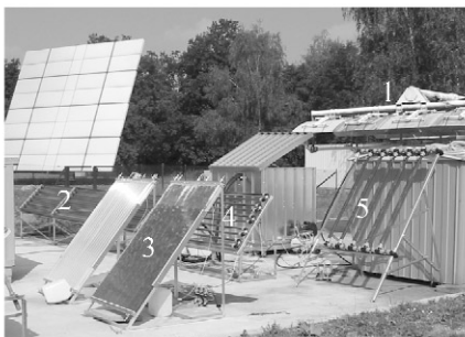
Fig. 5 Reactor comparison study (1: PROPHIS; 2: CPC; 3: flat bed; 4: horizontal tube reactor; 5: vertical tube reactor).
