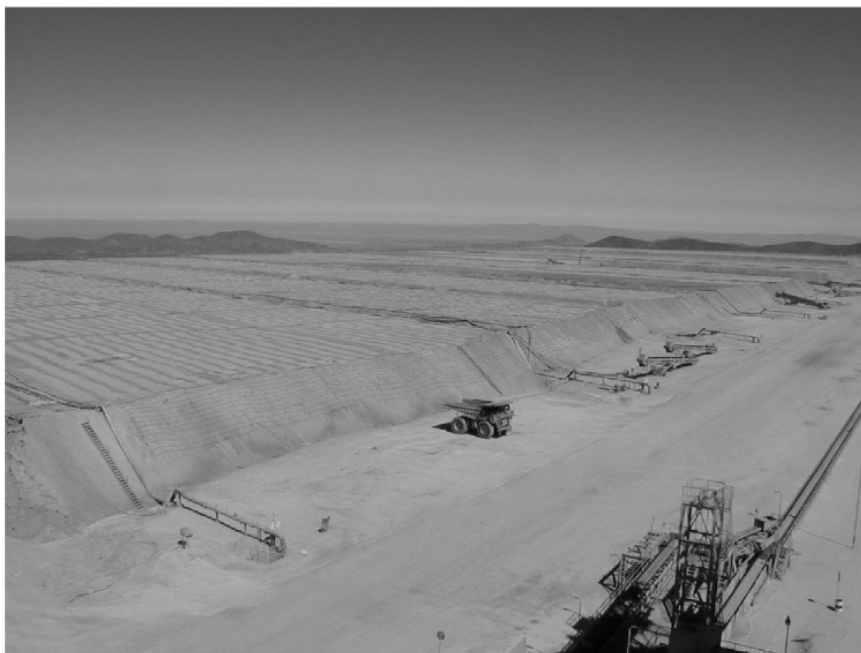
Fig. 3 Photograph of the copper heap-leaching operation at Cerro Colorado, Chile. Heaps of copper-containing mineral have been stacked, an irrigation system has been placed on top of the heap, and air is blown into the heap from below. The heap has been covered with an insulation thermofilm to reduce heat loss. (Photo courtesy of Rodolfo Reyes via Chris du Plessis.)
