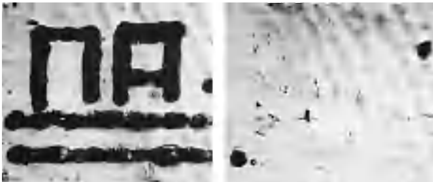
Fig. 13. Polymeric film in illuminated light: a - transparent film with the laser-recorded letters, b - this film after applying an electric field.
