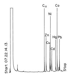
Fig. 4. Capillary gas-chromatogram of trifluorethyldithiocarbamates after extraction from aqueous solutions (see text). Metal contents of aqueous solution: Zn, Cu, Ni, Co-5 ppb, Cd-10 ppb, Hg, Pb-20 ppb. GC-conditions: 20 m SE 54, 70 - 240°, 8°/min, 2 µl splitless injection, FID-He. C.f. (41). <u>Acknowledgement</u> - This work was supported by grants of the Deutsche Forschungsgemeinschaft und Verband der Chemischen Industrie (BRD).
