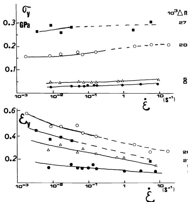
Fig. 10: Yield stress and strain of uniaxially drawn films as a function of elongation rate; discontinuous lines correspond to rupture without yielding.
