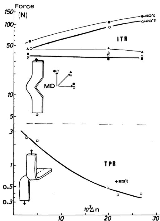
Fig. 22: Initial Tear Resistance and Tear Propagation Resistance of uniaxially drawn films versus birefringence along the direction of tear propagation (MD). Participants 2 and 3.
