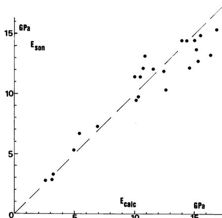
Fig. 9: Sonic modulus of uniaxially drawn films (drawing temp. between 100° and 160°C) versus calculated modulus based on two-parameter model (Eq. 2). Data from Participant 6.
