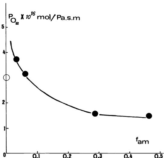
Fig. 30: Oxygen permeability of uniaxially drawn films as a function of non-crystalline orientation. Data from Participant 1.
