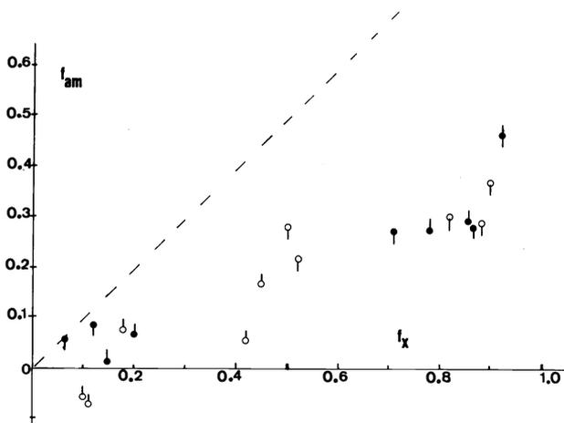
Fig. 1: Non-crystalline versus crystalline orientation in uni- and biaxially drawn films:
