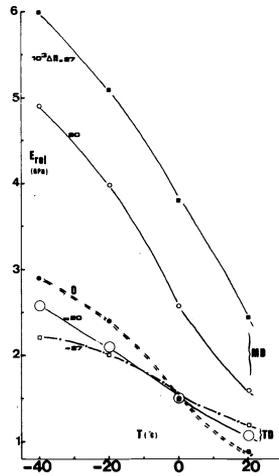
Fig. 5: Relaxation modulus at 100 seconds and 1% elongation for isotropic and uniaxially drawn films, measured in M- and T-directions at different temperatures. (Participant 5).
