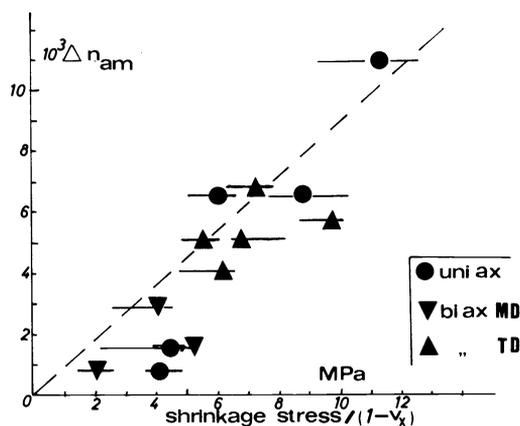
Fig. 29: Non-crystalline birefringence in uni- and biaxially drawn films versus shrinkage stress in amorphous phase. Comparison with stress-optical law for molten polypropylene. (Ref. 20). Experimental data from Participants 1, 4 and 6.
