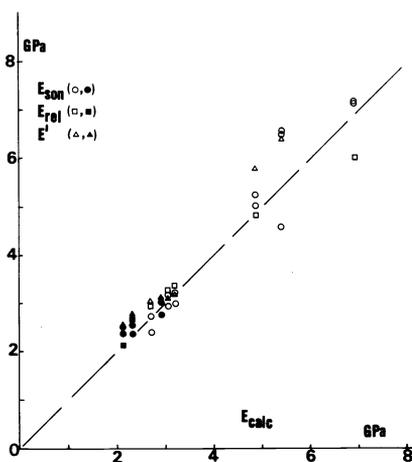
Fig. 8: Experimental relaxation, storage and sonic moduli of uniaxially drawn films versus calculated moduli, deduced from a two-parameter model. Data from Participants 3,4,5 and 6: open symbols: MD; closed symbols: TD.
