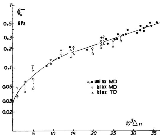
Fig. 16: Rupture stress of uni- and biaxially oriented films as a function of birefringence (elongation rate from  $10^{-2}$  to  $20\text{s}^{-1}$ ). Participants 1, 4 and 6.
