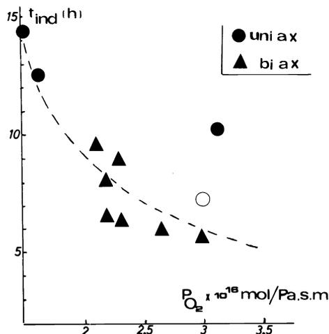
Fig. 31: Induction time (UV-stability) at 70°C (1 atm O<sub>2</sub>-pressure, light intensity = 885 W/m<sup>2</sup>) for uni- and biaxially drawn films (Participant 5) plotted versus O<sub>2</sub>-permeability measured by Participant 1.
