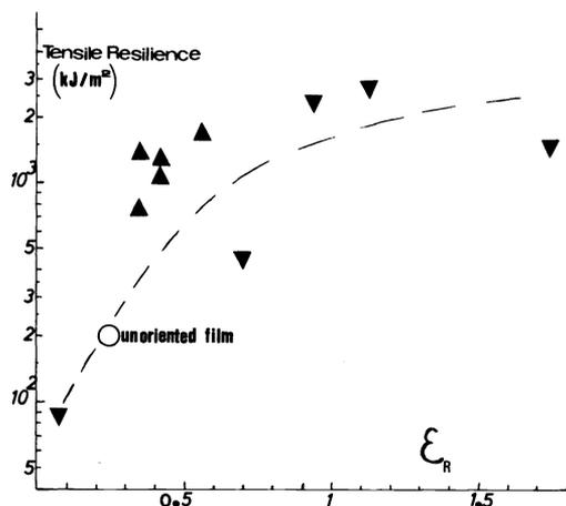
Fig. 21: Tensile resilience in M- and T-directions of biaxially oriented films versus rupture strain (measured at  $10s^{-1}$ ).
