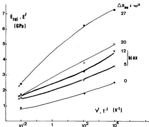
Fig. 4: Frequency dependence at room temperature of tensile storage or relaxation modulus of uni- and biaxially drawn films. Tensile stress parallel to M-direction.
