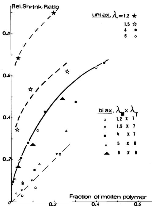
Fig. 28: Relative shrinkage ratio (Participant 1) versus fractional melting peak area (Participant 3) between 110° and 160°C, for uni- and biaxially drawn films.
