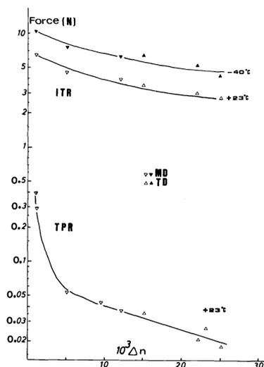
Fig. 23: Initial Tear Resistance and Tear Propagation Resistance of biaxially oriented films versus birefringence along the direction of tear propagation (either MD or TD). Participants 2 and 3.
