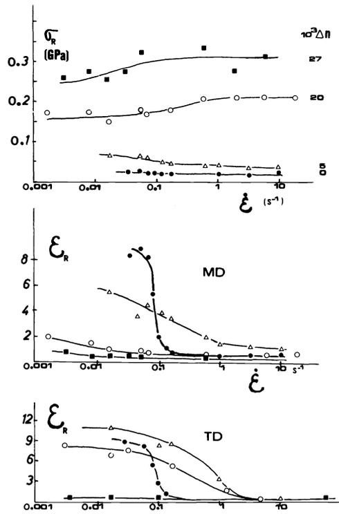
Fig. 13: Rupture stress and strain of uniaxially drawn films as a function of elongation rate (Participant 1).
