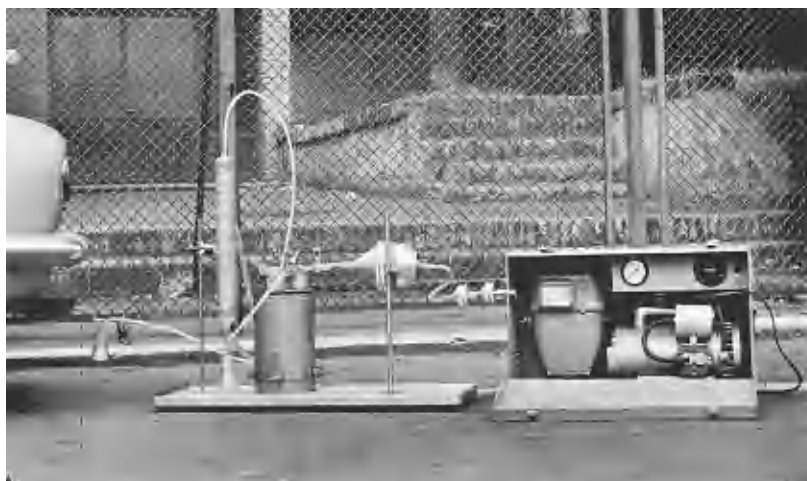
Figure 2. Engine exhaust sampling apparatus for determination of polycyclic hydrocarbons.
