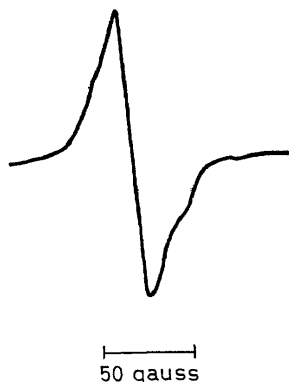
Figure 4. Electron spin resonance spectrum of poly(2,5-dichlorostyrene) irradiated at 300°K and observed at 300°K, after Florin, Wall and Brown 4
