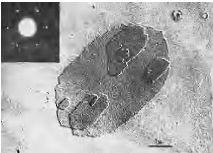
Figure 18. Electron photomicrograph of single crystal of trans -1,4-polybutadiene prepared from benzene solution at 18°C and its electron diffraction pattern
