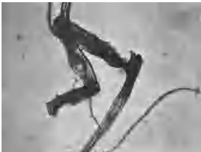
Figure 13. Microscopic examination of the fibre showing ruptured fibres
