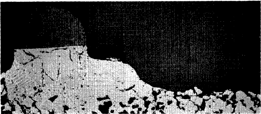
Figure 8. Micrograph of polycrystalline MgO sphere on top of polycrystalline \text{Fe}_2\text{O}_3 plate: humps in the spinel region at the \text{Fe}_2\text{O}_3 side are due to oxidation of spinel of intermediate composition the reaction layer; pores are created by the loss of oxygen at the spinel/ \text{Fe}_2\text{O}_3 . in Magnification 48.5\times (reduced by a factor of 0.6 in reproduction)
