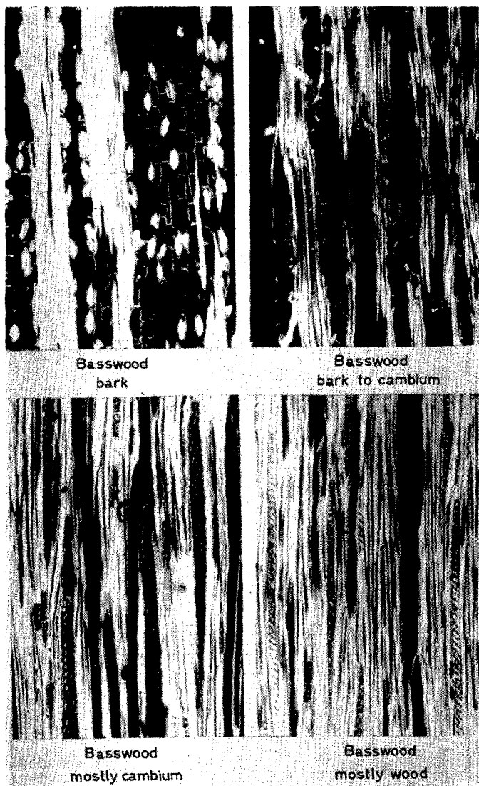
Figure 15. Photomicrographs of members of a series of tangential sections of basswood taken from bark → mature wood
