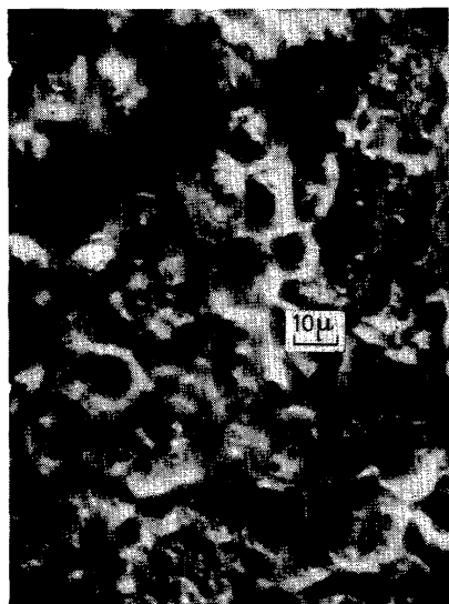
Figure 19. Low-density polyethylene subjected to slow cooling from the melt
