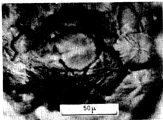
Figure 21. Spherulites of polypropylene, obtained by annealing at 130–140°
