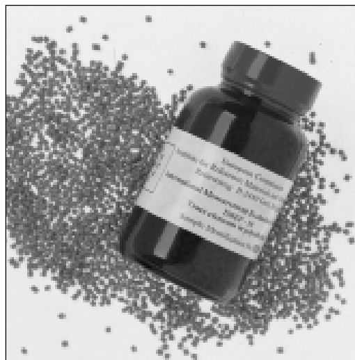
IMEP-10 bottle for the determination of Cd, Cr, Hg, Pb, As, Cl, Br, and S in polyethylene.
